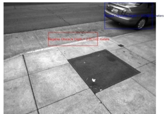
Figure 9. detecting both positive and negative obstacles
